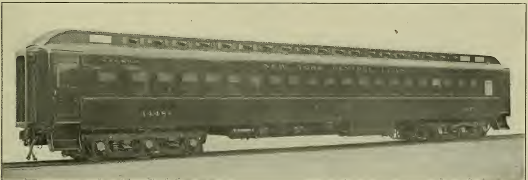
70-Ft. Steel Passenger Coach for the New York Central Lines.
